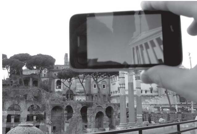
Figure 1. The application in use. Testing of the Forum Iulium sitsim on-site revealed that GPS positional error made the representation align improperly to reality, as expected. The temple should have been more to the left, in order to align to the real columns
